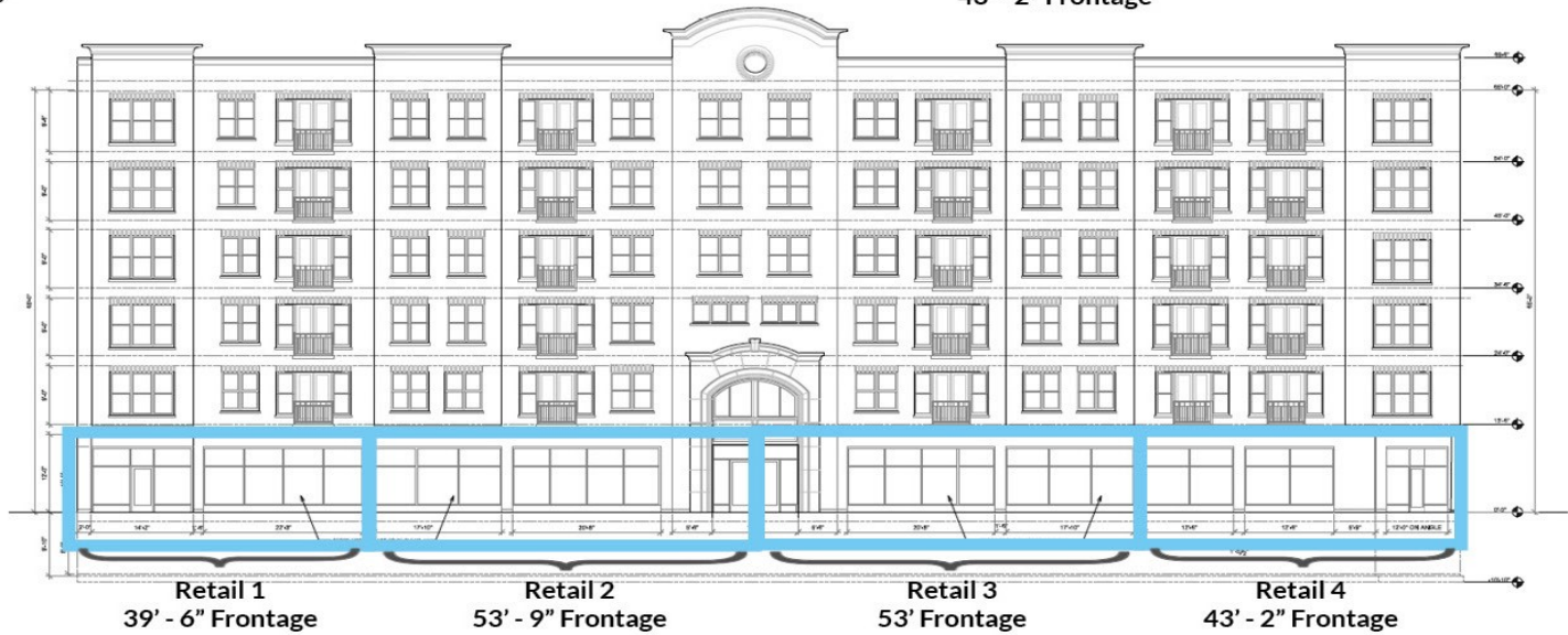
SOUTH ELEVATION (Milwaukee Ave) SCALE: 1/8"=1'-0"
